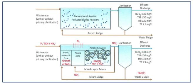
Use of SCR media in modified aeration basin allows for efficient nitrogen control. Adding a post-denitrification step can reduce total nitrogen even lower, to below 3 mg/l.
