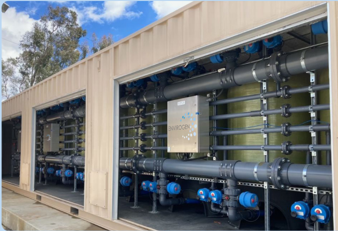
Envirogen's SimPACK (Left) and MinX (Right) regenerable IX systems, delivered as a containerized solution.
